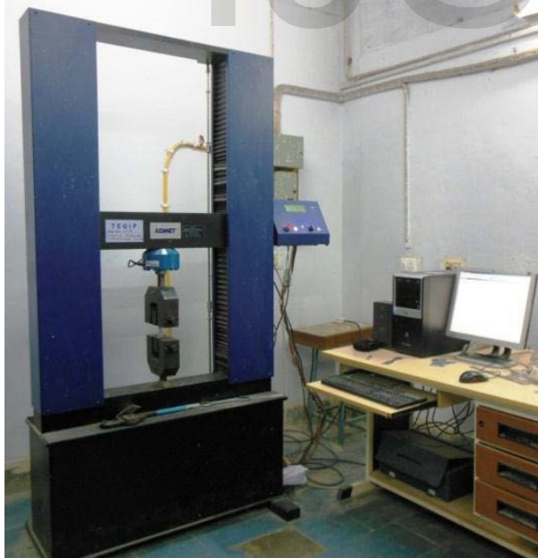
Fig 1. Specimen loaded on Universal Testing Machine
